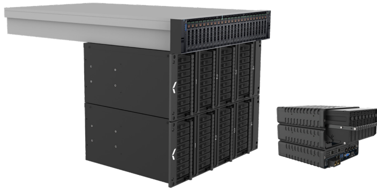
Fig. 2: Ingest station and in-vehicle data logger, concurrently collate 8 cassettes of data per server
