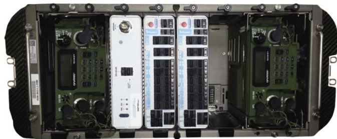
Figure 1 Multiple AN/PRC-117G radios mounted in a Voyager 8 chassis using two VoyagerMRBs
