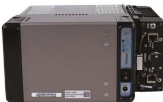
Figure 1: Voyager 2 rear showing UBI-2590 battery, DC input and HAIFE power
