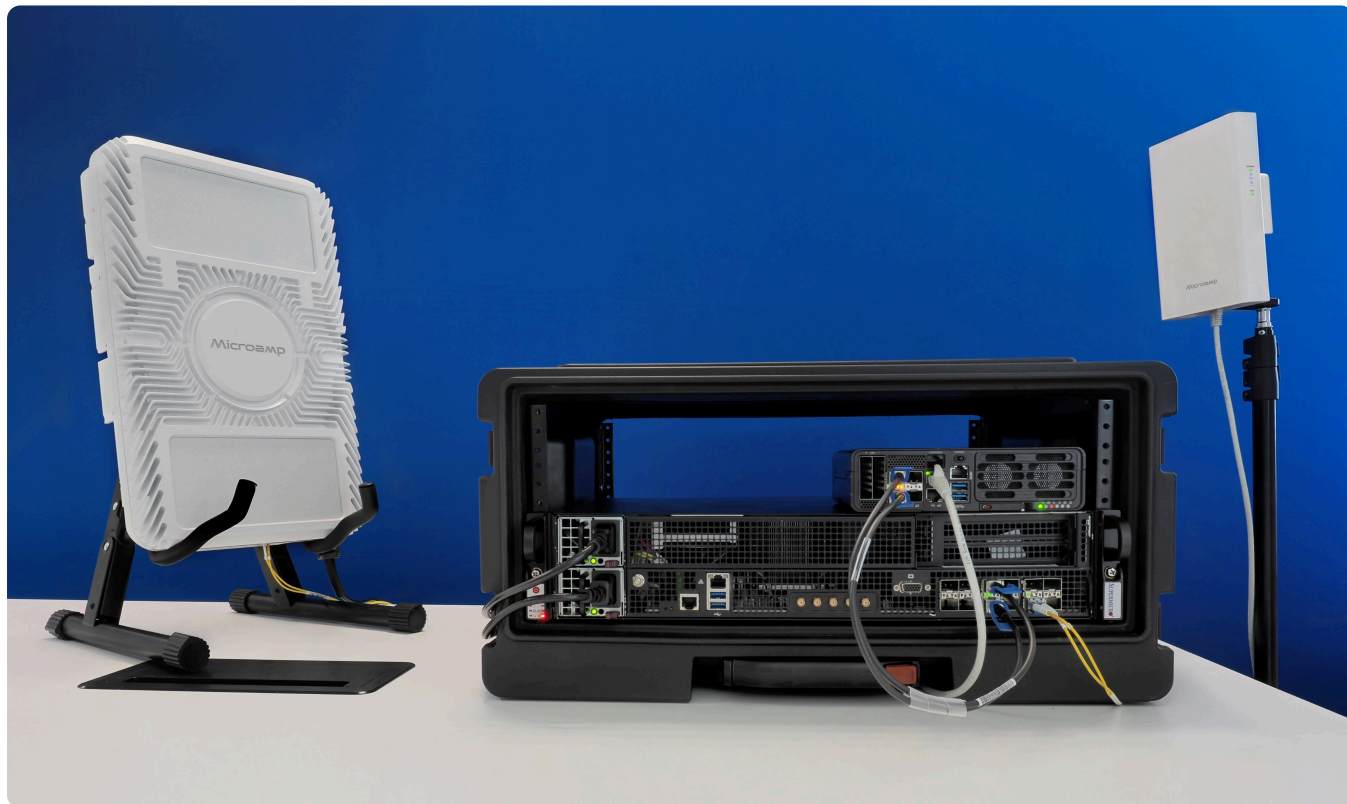
Fig. 2. Fully ruggedized setup used for the 5G mmWave Bubble deployment.
