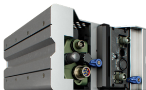
Harris Falcon III* AN/PRC-152A radio (dataport access) with an AR-20 or AR-20B amplifier. KLAS-VOY-RB24
