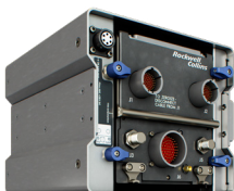
Single Aerospace Link 16 TacNet radio. KLAS-VOY-RB20
